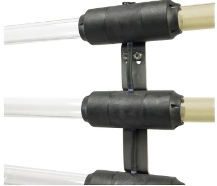
*UV lamps in TrojanUV systems are enclosed in a quartz sleeve to insulate them from the water. ActiClean™ is our patented dual-action sleeve cleaning system that uses mechanical wiping in conjunction with ActiClean Gel contained within wiper canisters surrounding the quartz sleeves.*
