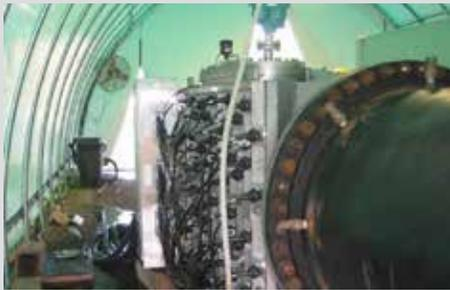
**Figure 2.** UV disinfection system undergoing performance evaluation through bioassay testing
