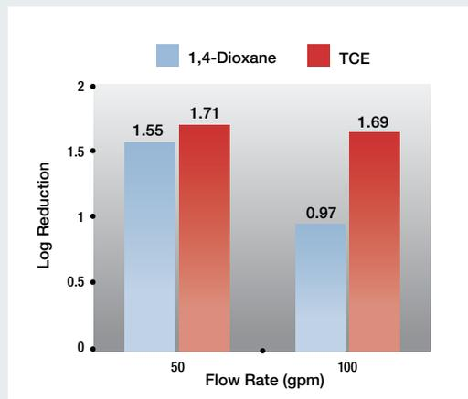
**Figure 1.** Results of pilot testing low-pressure UV-oxidation for treatment of indicated contaminants. Log reduction of contaminants treatment with UV-oxidation.  $H_2O_2$  concentration = 15 ppm.
