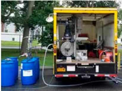
UV AOP pilot stations were easily transported between well sites, enabling the facilitation of over 24 separate pilots in six months.
